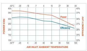
\* At ISO Conditions (59°F [15°C], sea level, 60% RH); high pressure natural gas Electrical efficiency tolerance: +1/-2.5 pts
