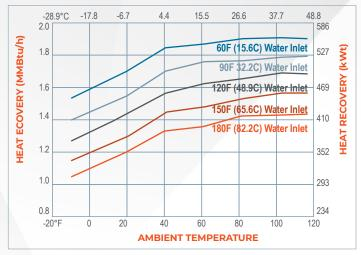
Note: Heat Recovery Unit (HRU) at 200 gpm (757 lpm) water flow, sea level, ± 15%
