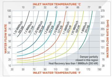
Note: Heat Recovery Unit (HRU) at ISO conditions, damper fully open, ± 15%
