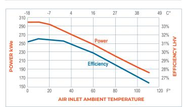
\* At ISO Conditions (59°F [15°C], sea level, 60% RH); high pressure natural gas \*\* Elevation derate of approximately 8.80 KW PER 1,000 FT (305 M)
