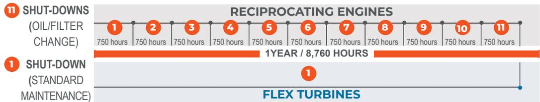
Flex Turbines require just one eight-hour period of scheduled maintenance per year. Overhaul of the Flex Turbine's prime mover is required just once every five to seven years. Reciprocating engines require shutdowns for maintenance every 750 hours and a top end rebuild every two years.
